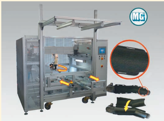
Fixing of acoustic capsules to plastic pipes
