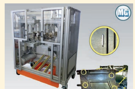
Attachment of aluminium sheets onto plastic panels
